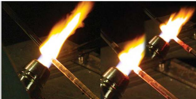
Puncture to sealed end of tube
