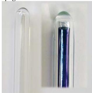
Seal one end of the tube and drop the dichroic in
